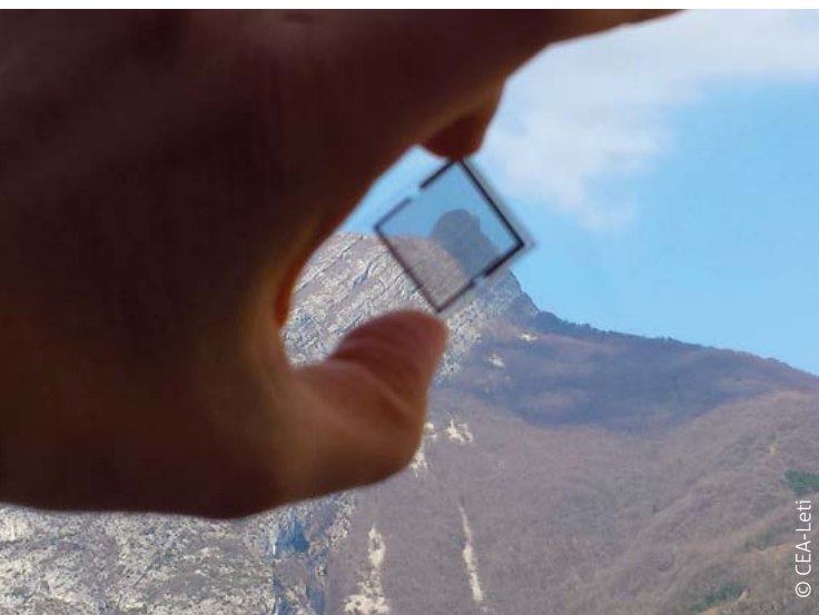
Actual photograph of a 25 × 25 mm² transparent thin-film battery (TFB).
